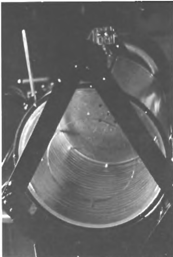
FIGURE 78. Rings forming in a liquid film attached to the inside wall of a rotating cylinder, as the cylinder is slowed down or suddenly stopped. (From Debler and Yih [1962], J. Aerosp. Sci. 29 , 364.)
